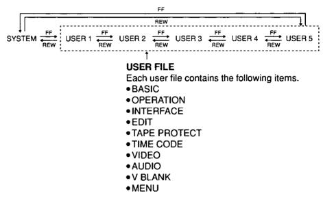
**3** Repeat the operation in step 2 to select the user file to be used and press the SET button. The user file is changed and stored in the memory.
